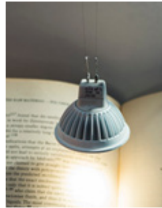
Carbon nanotube fibers support and power lamp
