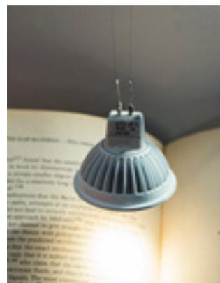
Carbon nanotube fibers support and power lamp
